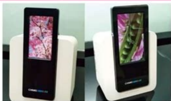
Fig. 1 features 3.4-inch and 4.3-inch TRUEOLED display, supporting over 300 ppi resolution, utilize top emission white OLED with color filter in RGBW pixel layout, to be manufactured without utilizing precision mask for EL deposition that provides advantages in terms of simple production process, low cost and high yield.
